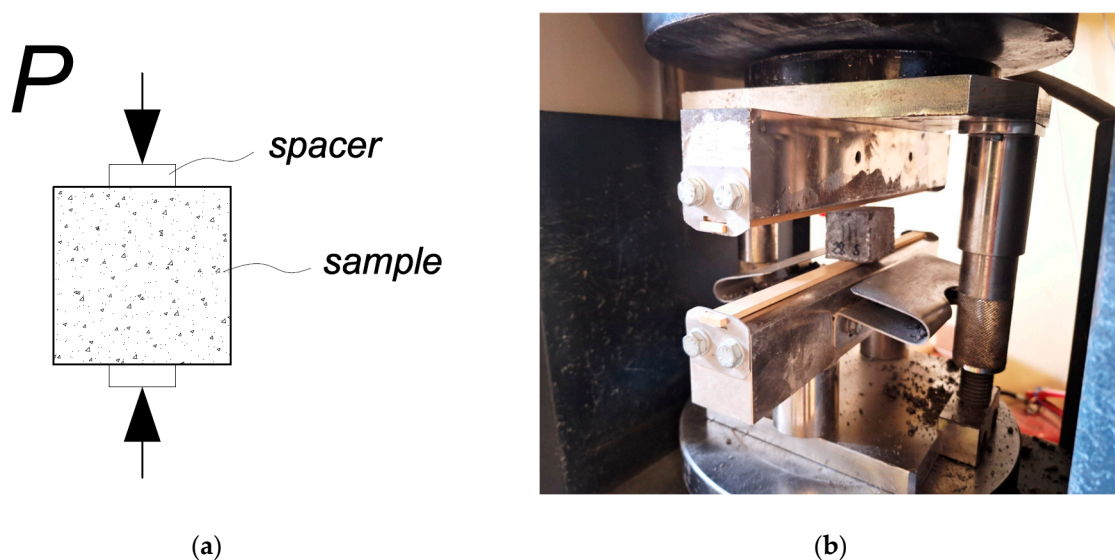
Figure 8. Drawing of the sample tensile splitting test scheme (a) and sample testing (b).
