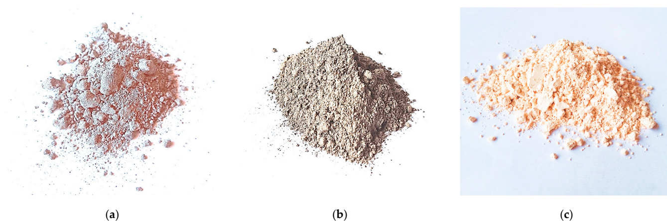
Figure 1. (MSWI) samples of bottom ash before milling (a) and after milling (b), Metakaolin waste (c).
