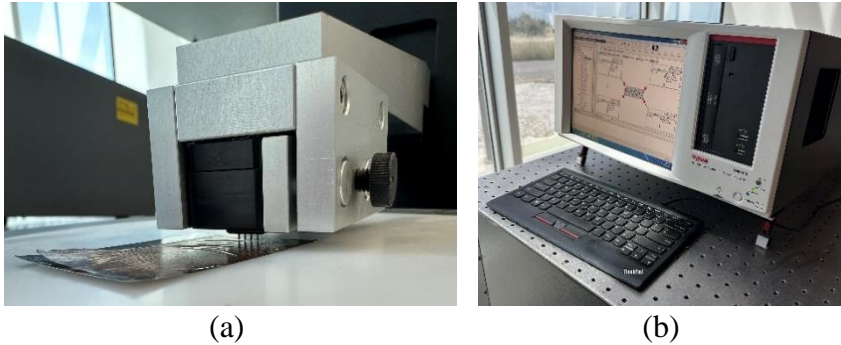
Fig. 2.12 The four-point probe method measuring equipment: (a) specimen measurement; (b) Model 4200-SCS Semiconductor Characterization System
