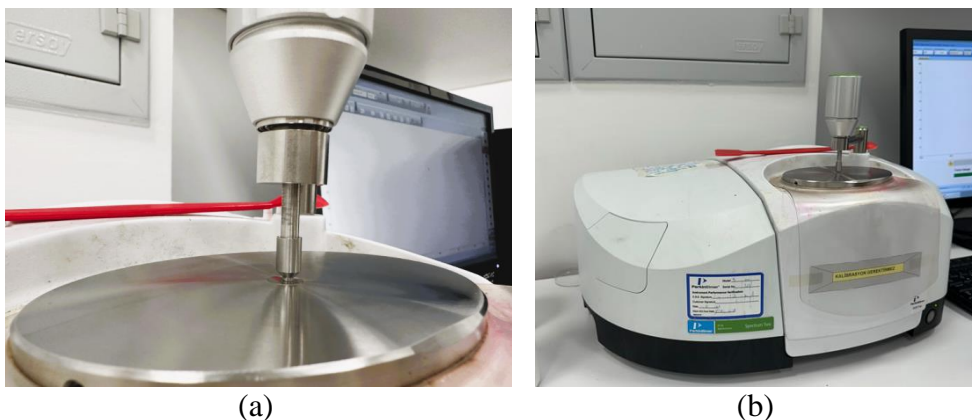
Fig. 2.1 FTIR measurement: (a) measuring of sample; (b) spectrometer
