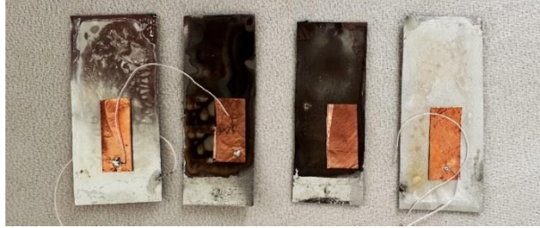
Fig. 2.9 Samples prepared on steel plates coated with different PVDF materials with a conductive copper phase on top and contacts
