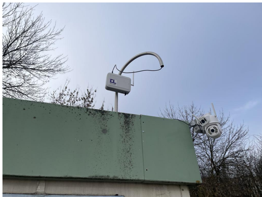
Fig. 8. A low-cost sensor mounted on an Environment Agency monitoring station
