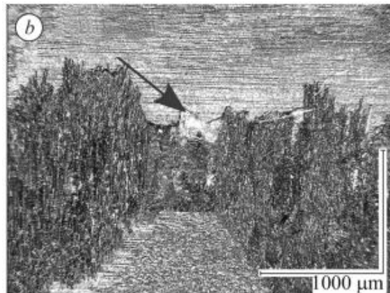
Fig. 8. Chipping occurring at the interface between the matrix and fibers is indicated by arrows [21]
