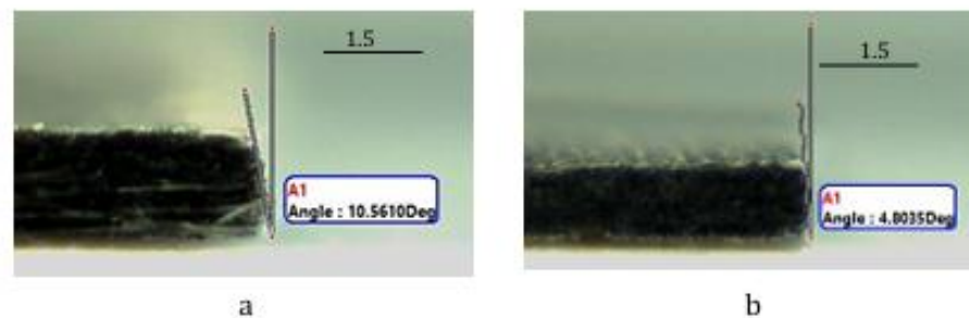
Fig. 5 The kerf angles of BFRPC: a - coarse cutting and b - fine cutting
