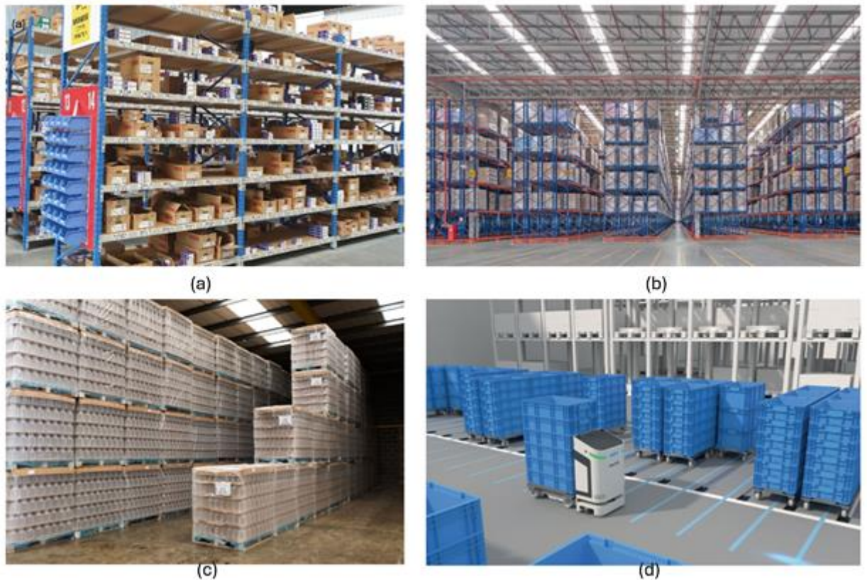
Fig. 8. Storage types in company “X”: a. bin shelves, b. pallet racks, c. pallet bulk store, d. trolley lanes [37,38,39 ,40]
