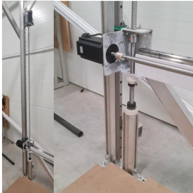
Fig. 25. Assembled Z-axis one corner
