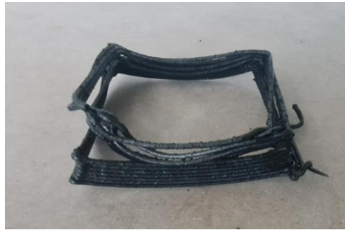
Fig. 41. Poor bed adhesion
