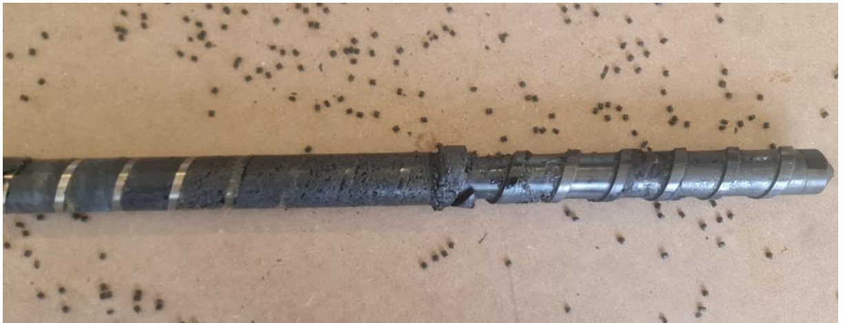
Fig. 36. Charred plastic around extruder screw
