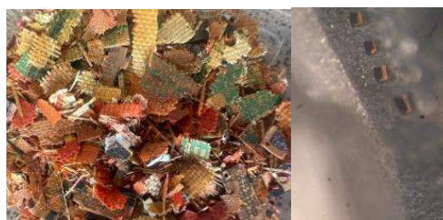
Figure 1: Figures illustrating the FR-4 residues after dissolutions of resins and hydrometallurgical extraction of metals. Gold residue is visible in the grooves of the processors plastic pieces.
