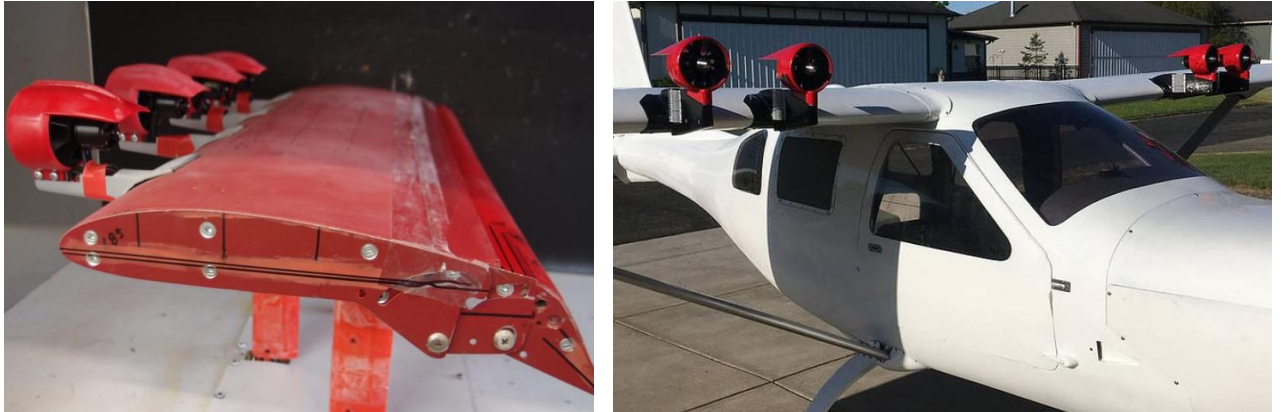
Fig. 13. JibirWatt EDF installation [36, 37]
