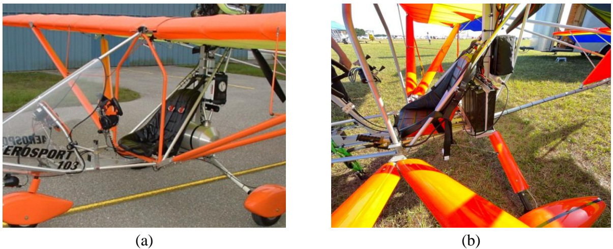
Fig. 16. Gas tank and battery location (a) Aerolite 103 (b) Aerolite EV-103 [19]
