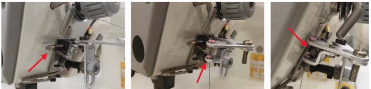
Fig. 22. Thread Tension Sensor Setup [24]
