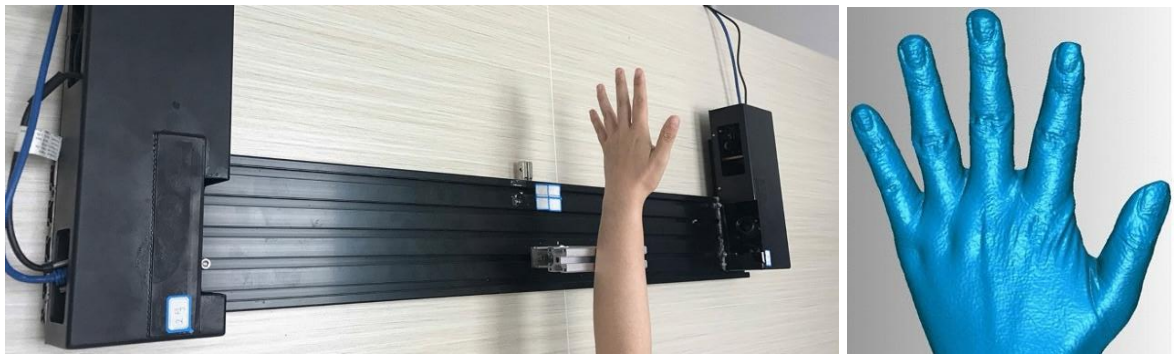
Fig. 6. Example of a Scanning System Where an Arm is Scanned from Both Sides Simultaneously [17]
