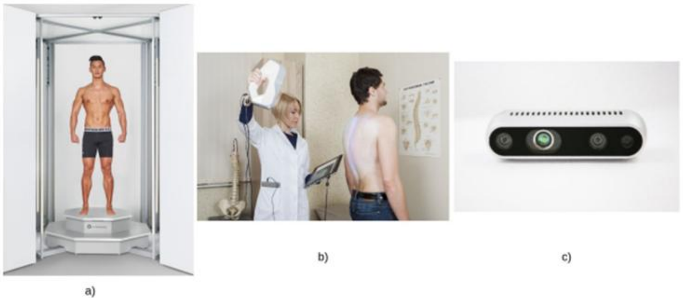
Fig. 3. Examples of Three Types of 3D Scanners in Terms of Their Scale [9]. Stationary (a), handheld (b) and mini scanners (c)
