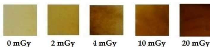
Figure 9. Change in the optical characteristics of PVA films, doped with NBT dye [67]
