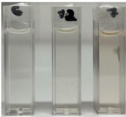
Figure 24. From left to right: pure PVA solution; S1 (0.45 w% \text{KIO}_3 ) solution 5 minutes post preparation; S1 (0.45 w% \text{KIO}_3 ) solution 15 minutes post preparation
