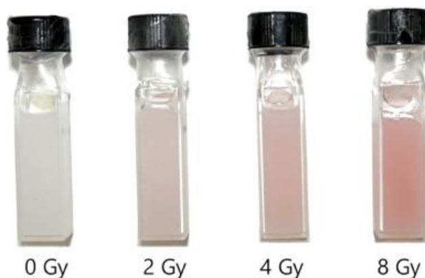
Figure 15. Color changes of PVA, iodide and silica nanoparticle containing indicator after irradiation to different doses [78]
