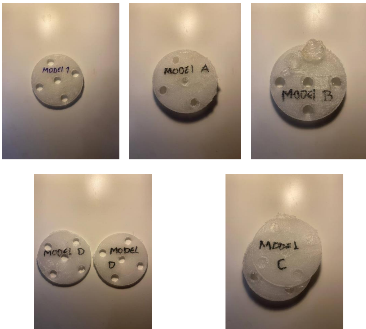
Fig. 24 Examples of 3D printed PMMA samples with 100% infill. All samples show material disruption at approximately 1.5-2 cm
