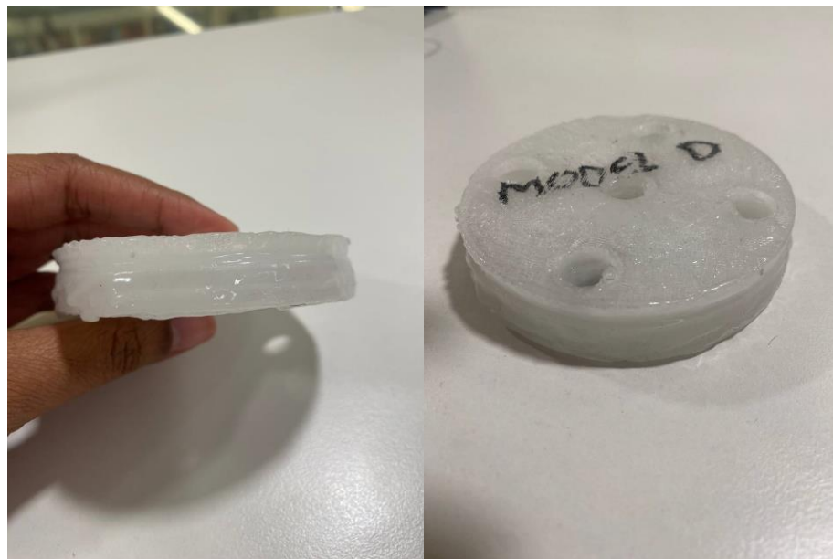
Fig. 11 Assembled phantom constructed by bonding individual PMMA printed discs using acrylic glue
