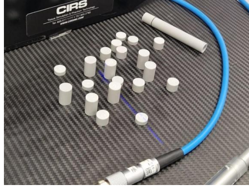
Fig. 21. Spacer plugs used for the ionisation chamber positioning
