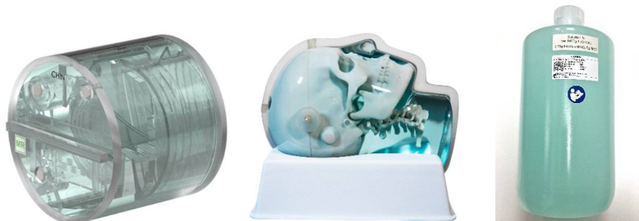
Fig. 9. Examples of MRI Phantoms: the Sun Nuclear ACR Accreditation Phantom [64] (left), used for standard image quality assessments; the Sun Nuclear SRS MR Distortion Phantom [65] (middle), designed
