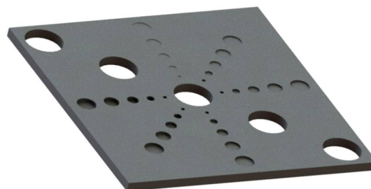
Fig. 23. Structure for low-contrast detection, which has five same depth cavities with ranging diameters
