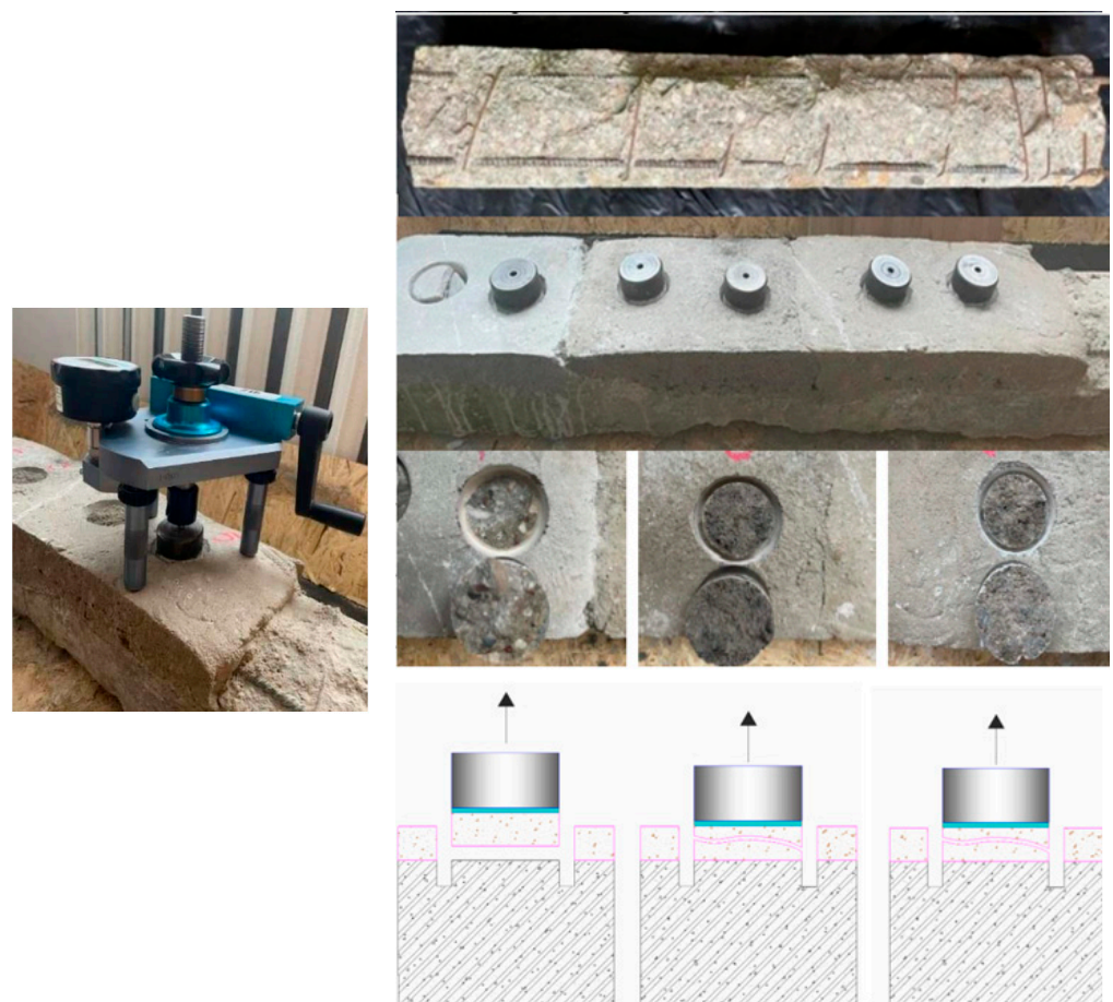
Figure 6. The old OPC concrete beam and visual identification of the type of failure according to a pull-off test (EN 1542) [21].
