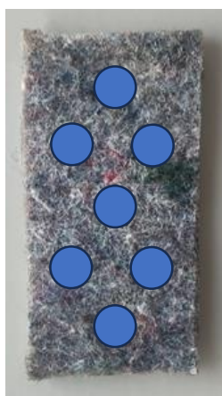
Fig. 1. Left – biofilter design. Points indicate areas where concentrated cell nutrient suspension was inlaid. Right – Bioaccumulation capacity of the tested filter. Initial Zn 2+ concentration – 53.15 μM.
