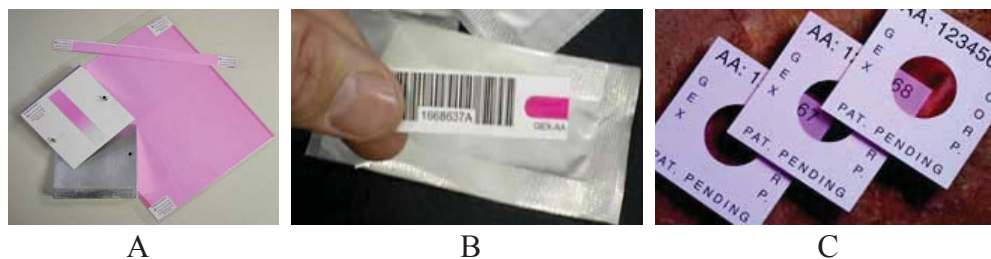
Fig. 11. A – irradiated Risø B3 film; B and C – GEX DoseStix and WinDose dosimeters made from Risø B3 film, respectively. (Adapted from Ref. [19]).
