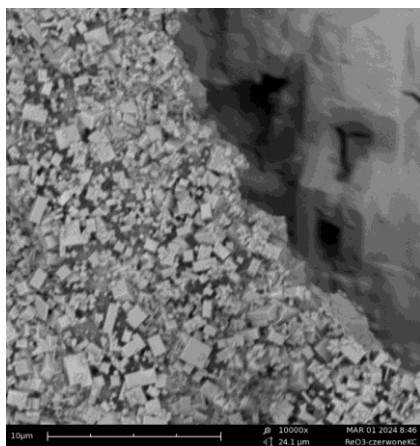
Figure 7.3.1 Scanning electron microscopy (SEM) image of rhenium trioxide crystals deposited onto a glass substrate through physical vapor deposition (PVD).
