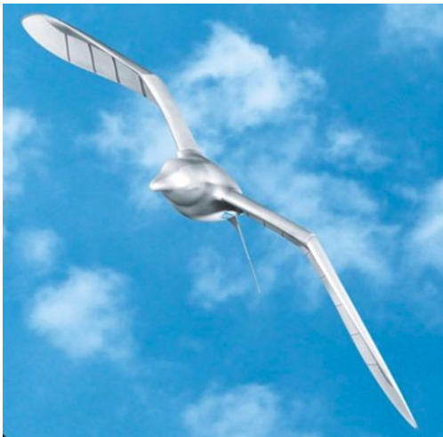
Figure 1.1.2. SmartBird flies like a bird (FESTO).
