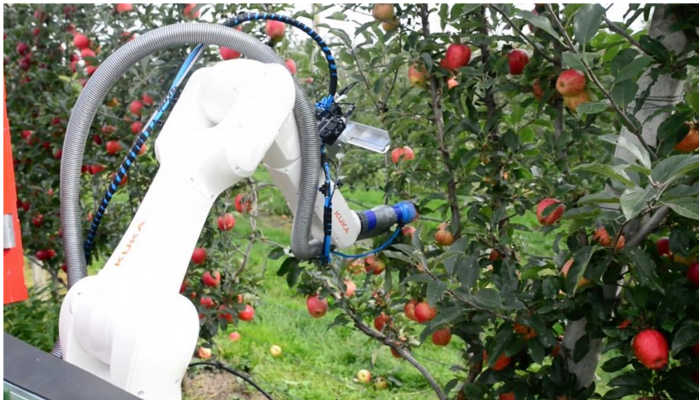
Figure 1.2.6. Pilot project - The KUKA CropBot has mastered its first harvesting operation. It gently sucks the apples from the tree – supported by a vision system (KUKA).
