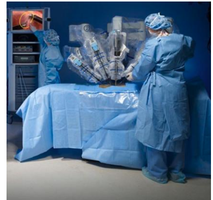
Figure 1.1.6. Da Vinci Diagnostic: This robot assists doctors with complex examinations and surgical procedures (INTUITIVE SURGICAL).
