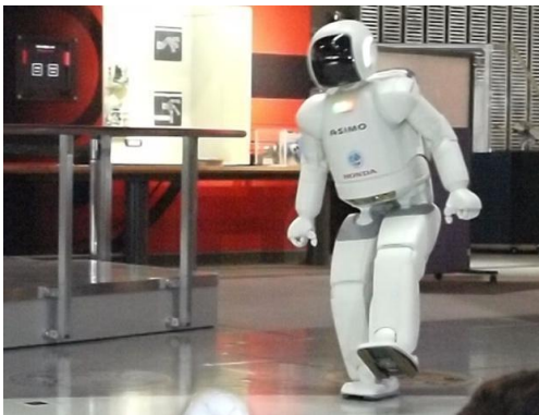
Figure 1.1.12. ASIMO shows the sole of the left foot which is part of the Floor Reaction Control (Wikipedia).
