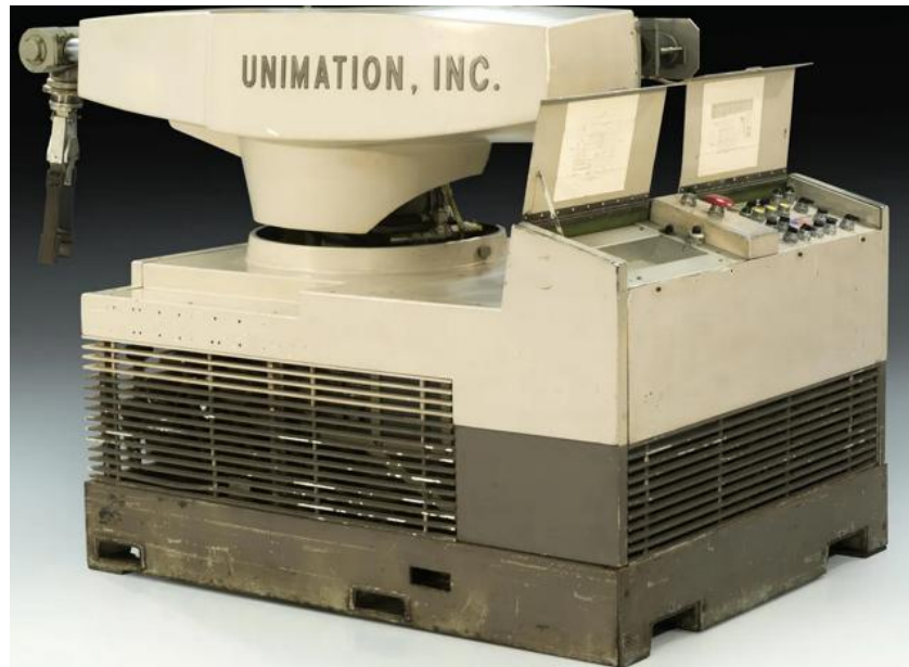
Figure 1.1.9. Unimate, the first industrial robot (IEEE Spectrum).
