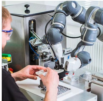
Figure 1.1.5. YuMi, human-machine collaboration robot (AB)
