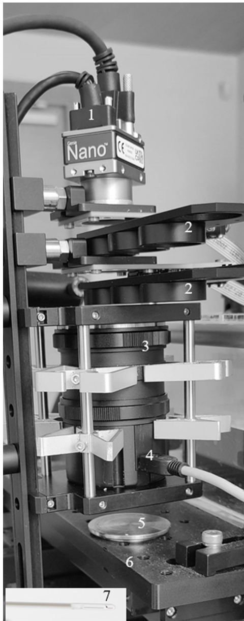
Figure 8. Proposed set-up for Raman+NIR-autofluorescence spectral band imaging implementation for veterinary clinics: (1) – M2590, 1" NIR camera (Teledyne Dalsa, Canada); (2) – two automated sliding filter compartments (Thorlabs, USA) equipped with calibrated rotation filters ( \varnothing 1" ); the proposed solution eliminated the manual rotation of two narrowband filters needed to apply during the measurement; (3) – macro imaging lens with magnification up to 5\times (Yasuhara Nanoha, USA), 4 – USB powered white light LED source; 5 – sample tray (Raman signal inactive); 6 – x-y-z translation stage (Standa, Lithuania). A low-cost fiber-coupled Raman laser (FC-D-785-450mW, CNI Optoelectronics Technology Co., Ltd, China) is used for Raman excitation via a 30-degree side-fire fiber probe (7), produced by Lightguide (Latvia). The probe is positioned with an additional tilting angle between the objective and tissue specimen, allowing 785 nm Raman excitation light to be delivered to the sample without interfering with the detection optics.
