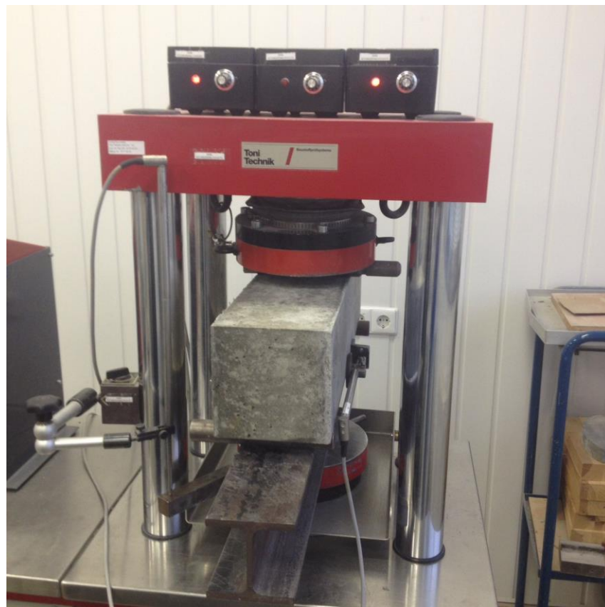
Figure 13 Image of specimen set up for three-point bending test from laboratory
