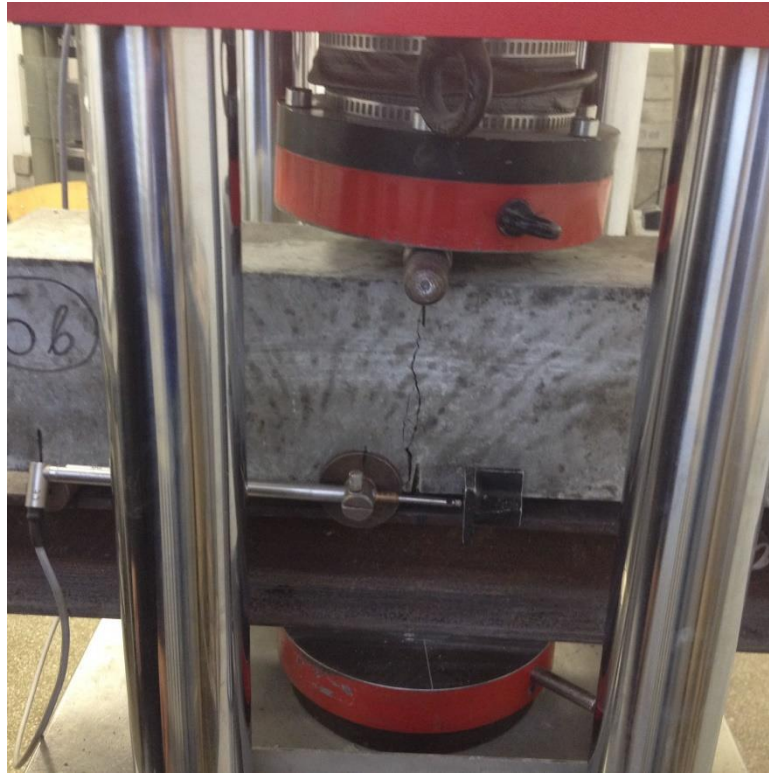
Figure 14 Image of specimen set up for three point bending test from laboratory
