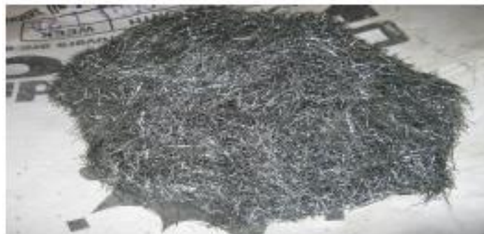
Figure 4 Schematic representation of steel fibres used in the above experiment
