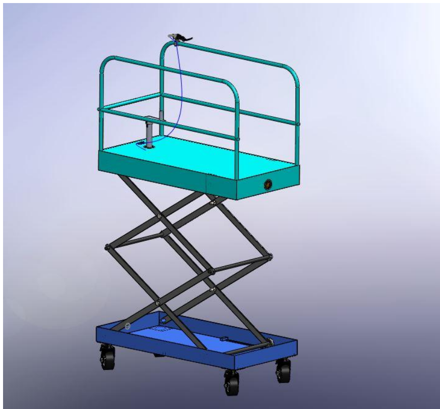
Figure 3.10. 2 Scissor lift at final position
