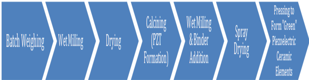
Figure 1-2 The Process of Manufacturing PZT [Source - APC International, 2016]
