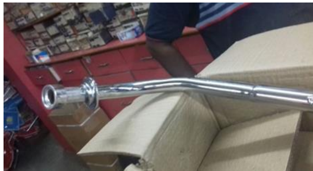
Figure 1 Zinc – Nickel coated exhaust pipe of mild steel
