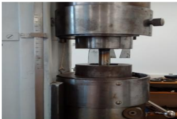
Figure 16 The specimen fixed in the tension-compression machine
