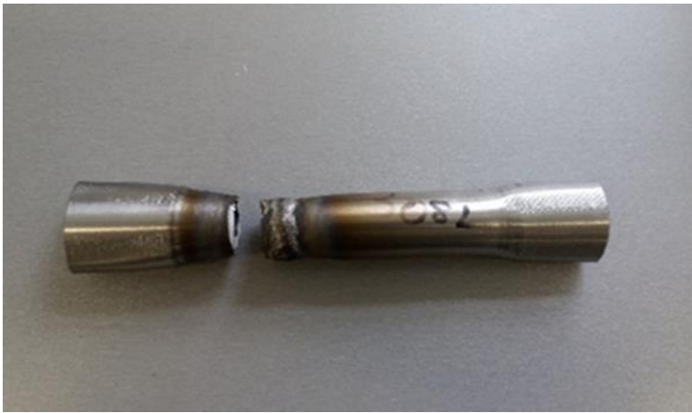
Figure 17 Specimen after the tensile test
