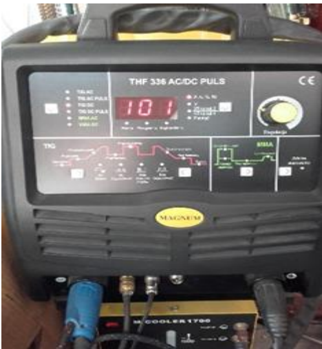
Figure 15 TIG welding machine used for welding
