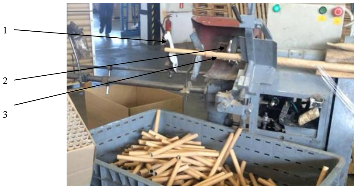
Fig.2.14. The cutting unit with a target 1 and circular saw blade 2 for cutting cardboard tubes 3
