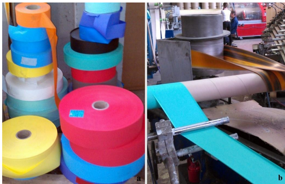
Fig.1.9. Variety of different papers used for: a) textile tubes and b) textile tubes winding principle
