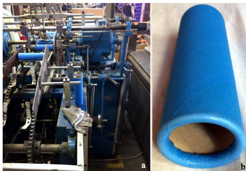
Fig.2.9. A view of: a) curling machine and b) inside-curved tube
