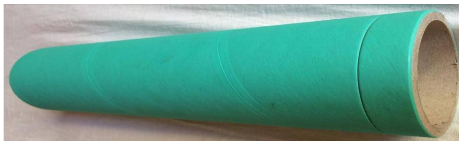
Fig.3.4. Special groove on a cardboard tube for securing string
