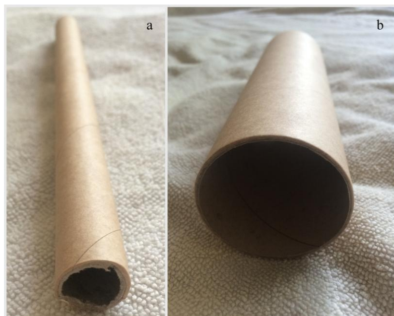
Fig.1.7. Cut edges of cardboard tubes: a) poor quality, b) good quality
