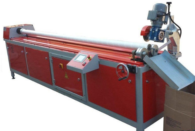
Fig.2.12. The UBR Paper Machinery Tube Re-Cutter Machine by Servo Cutting System [16]
