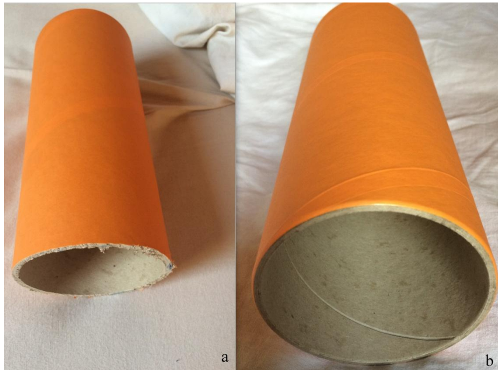
Fig.1.8. Cut edges of specialist tube: a) poor quality, b) good quality
