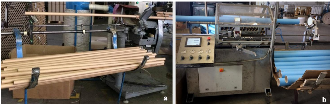
Fig. 5.4. Comparison of: a) original cutting mechanism and b) modernized cutting mechanism
