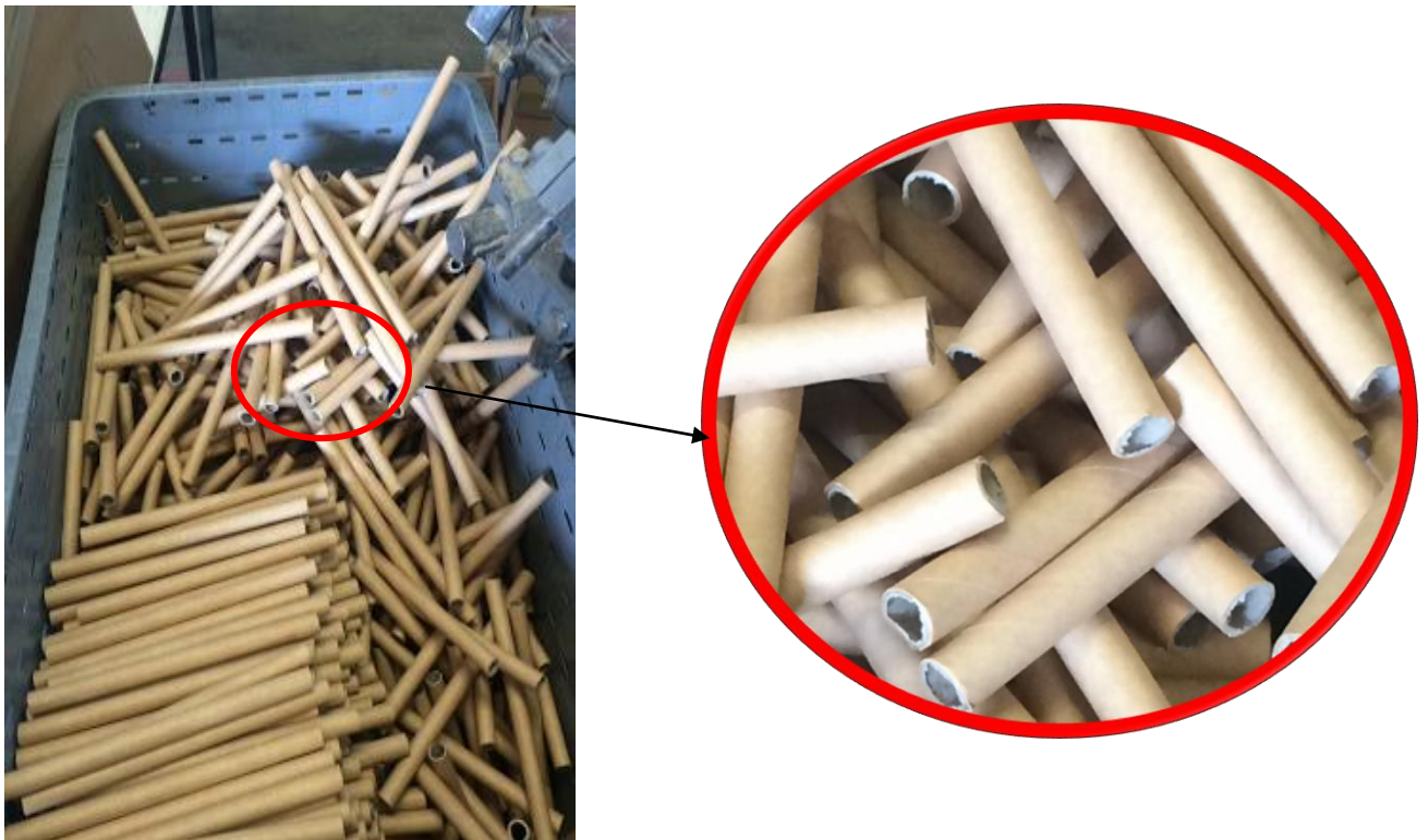
Fig.2.15. The quality of cut cardboard edges
