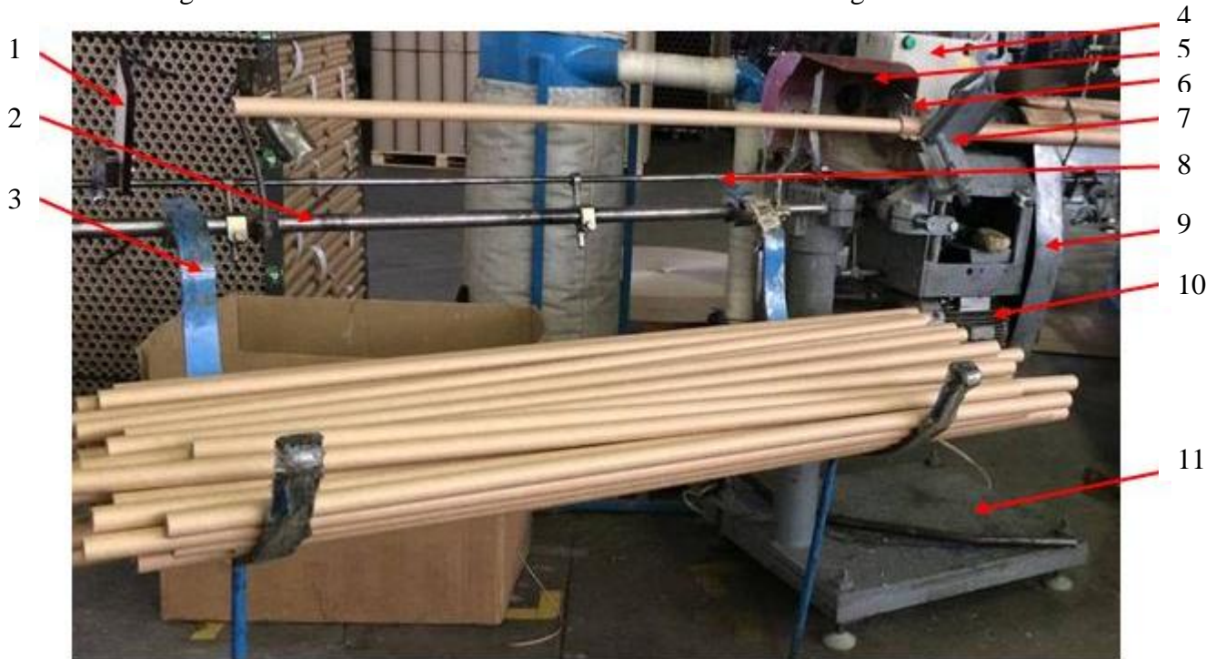
Fig.3.1. Original cutting unit with target 1 , supporting rod 2 , frame 3 , control board 4 , cover 5 , circular saw blade 6 , chuck 7 , pneumatic cylinder 8 , cover 9 , motor 10 , stand 11
