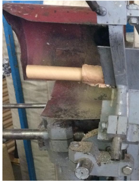
Fig.3.3. Dusts on the cutting mechanism
