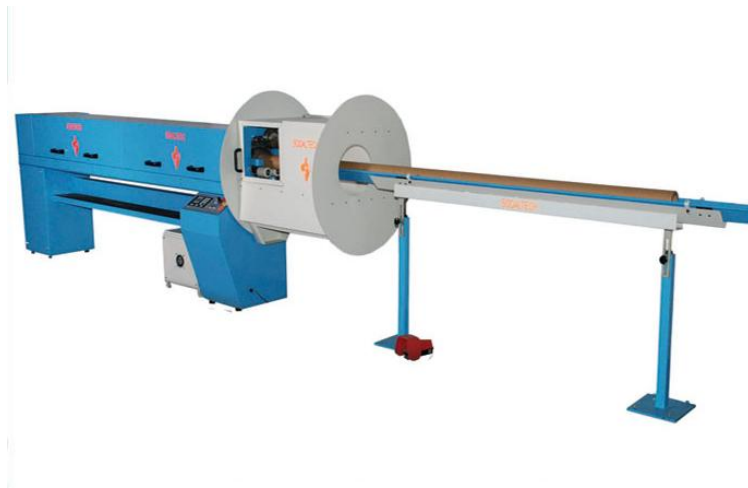
Fig.2.11. The “Sodaltech” Automatic Core Cutter [15]
