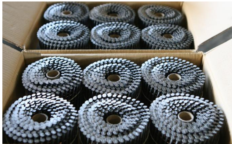
Fig.1.6. Spiral cardboard tube used for packing wire coil nails [12]
