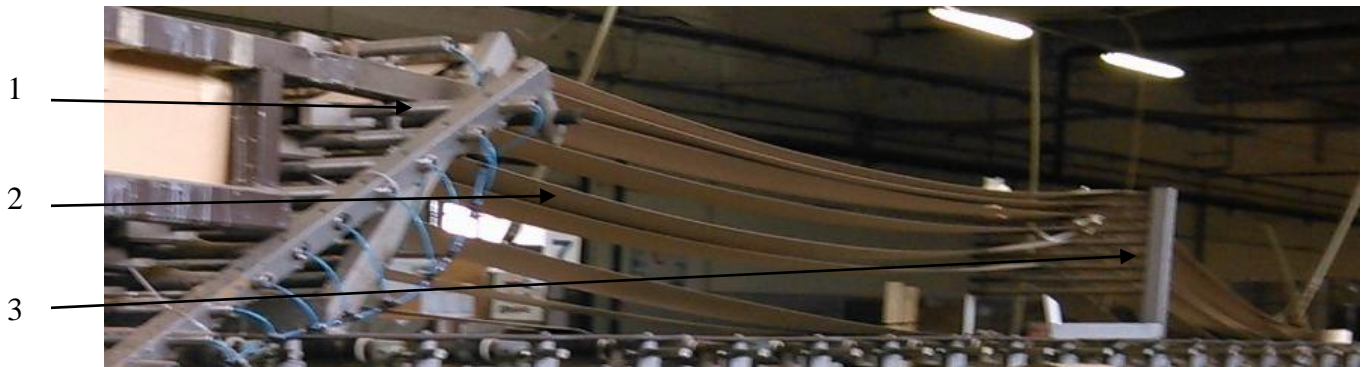
Fig.2.4. Stretching and retaining system with paper stretchers 1, paper plies 2 and paper retainers 3
