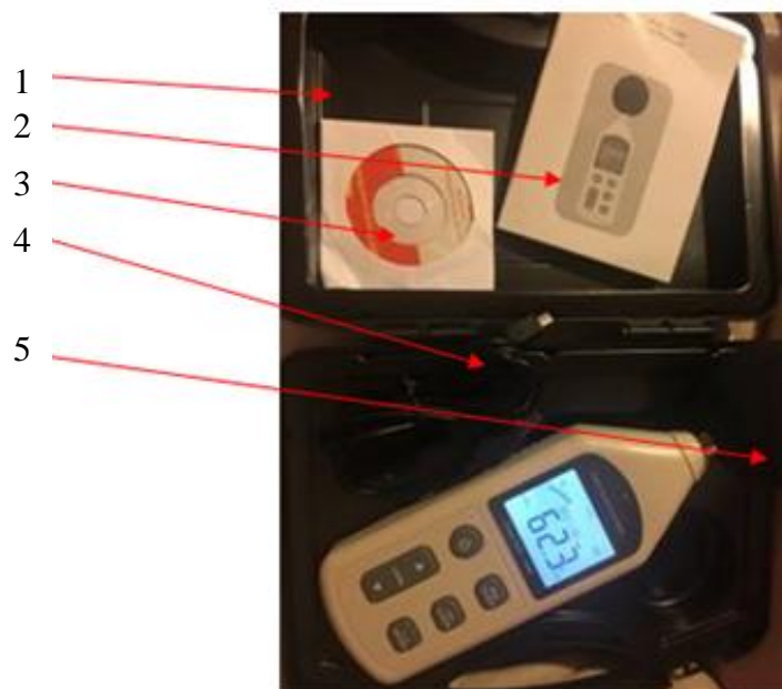
Fig.5.3. Sound Level Meter FRA-1356 with transportation case 1, manual 2, software CD 3, USB cable 4 and protective sponge ball 5
