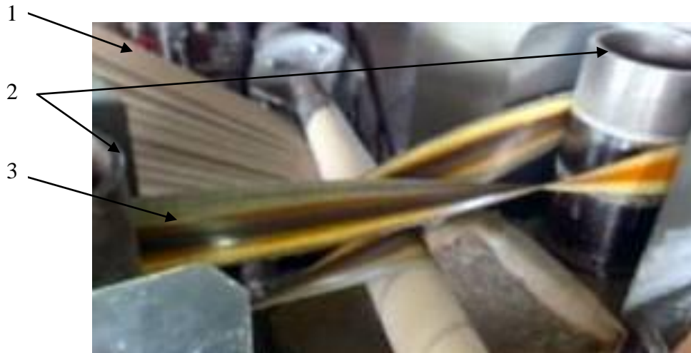
Fig.2.6. Cardboard plies winding mechanism
