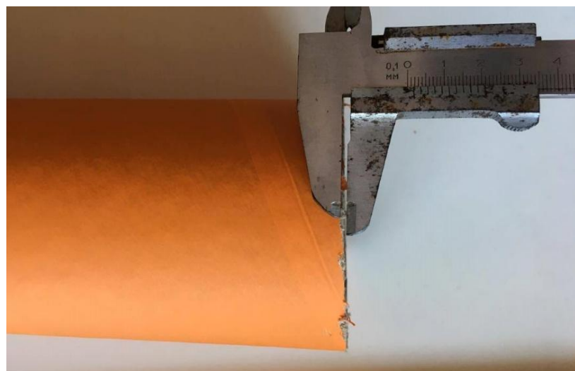
Fig.3.2. Rips, burrs and jags on cutting edge
