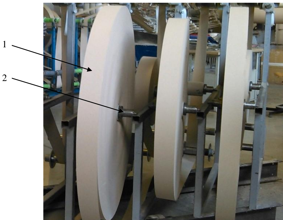
Fig.2.3. Cardboard roll 1 onto revolver winder 2
