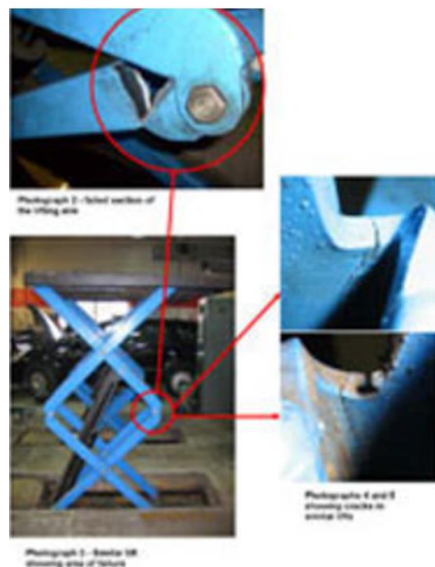
Fig 9. Wear and fracture in joints [47]
