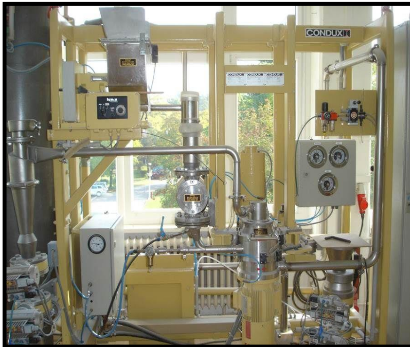
Figure 7: Condux Fractionation System (IGV)
