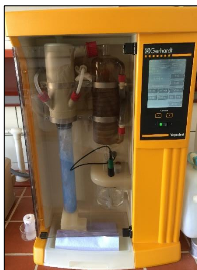
Figure 14: Gerhardt Kjeldahl apparatus used for analysis of crude protein in test samples at IGV
