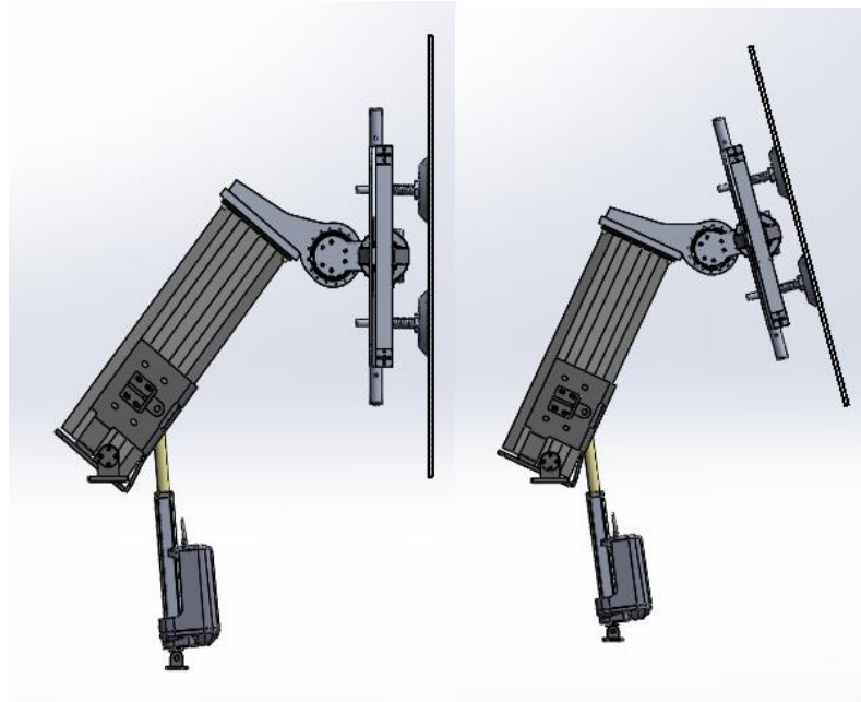
Fig. 3.2 The vertical hold and 30 degree hold position. Gripper holds the glass in vertical position for further transportation
