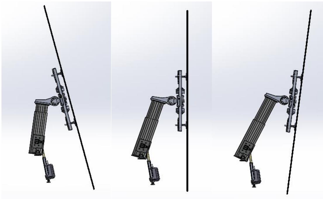
Fig. 3.6 30 degree, vertical and installation hold positions. The glass is prepared to be inserted into the frame
