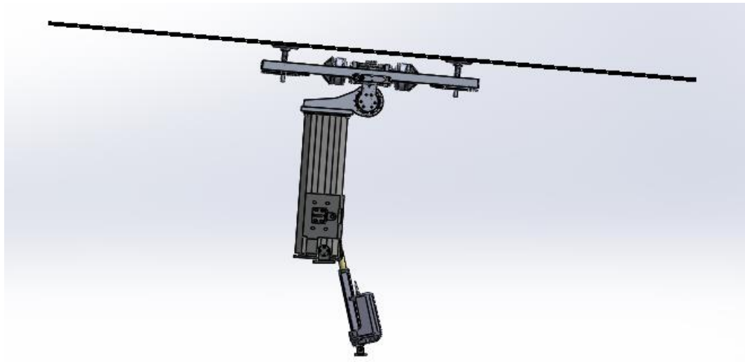
Fig. 3.4 The transportation-ready position of co-bot. The glass panel was turned manually to vertical position
