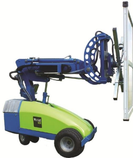
Fig. 1.3 The Winlet 600 glazing robot made by the Winlet Company. [3]
