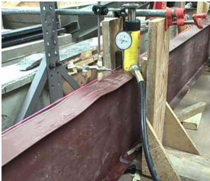
Fig. 1 Hydraulic jack to remove the flange bends [1]
