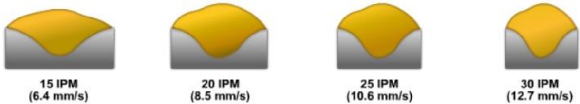
Fig.9 Difference in weld beads for different travel speeds (source: weldguru.com)
