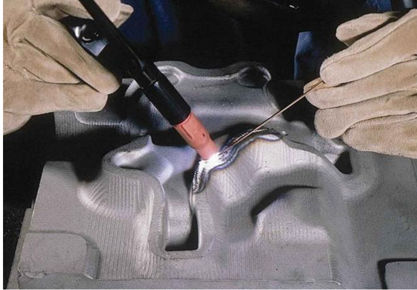
Figure 5 Gas tungsten welding example
