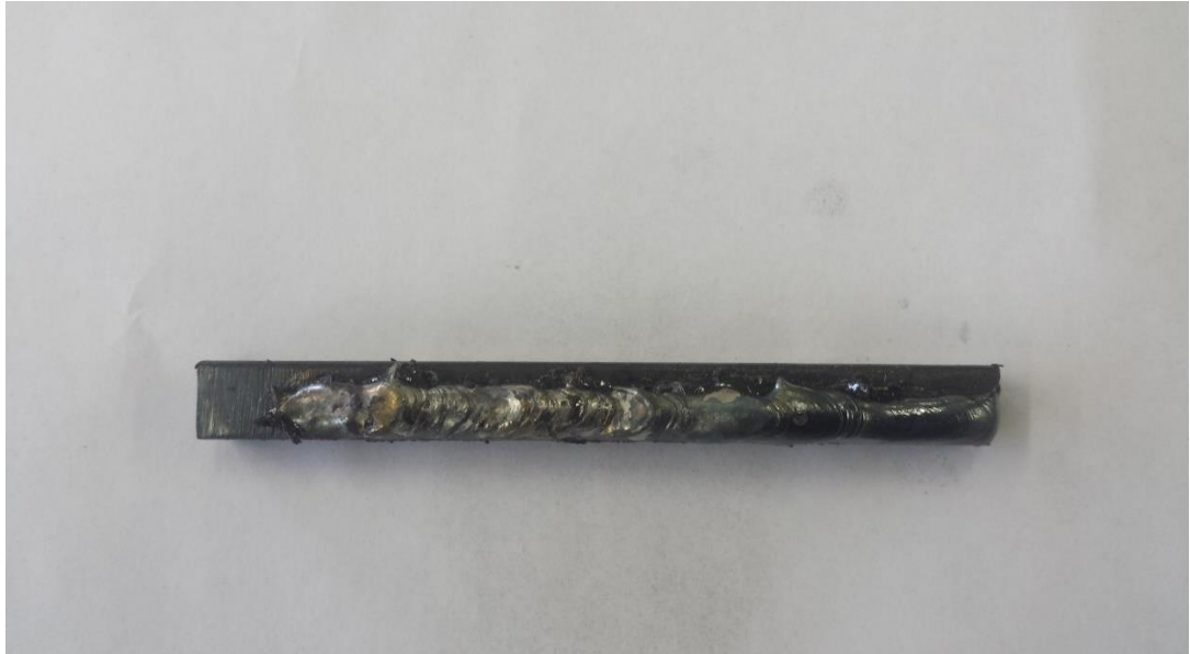
Figure 15 Sample output after welding
