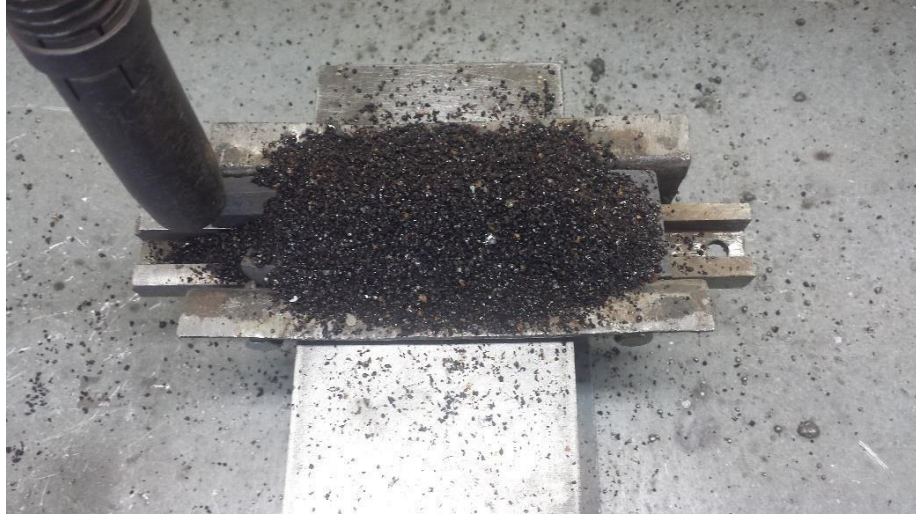
Figure 13 Mixture of both Hard and self-fluxing powder
