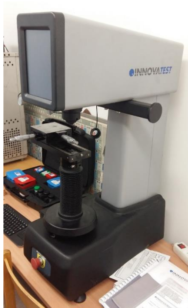
Fig. 2.14. Hardness testing instrument Inovatest Verzus 750ccd
