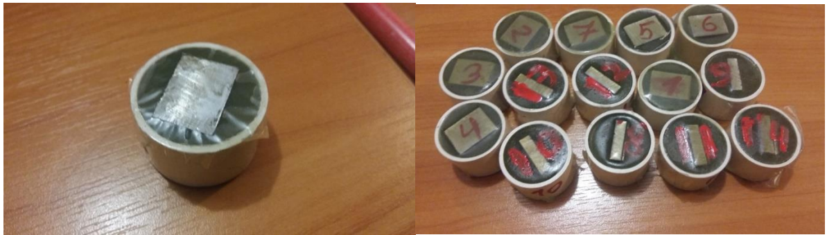
Fig. 2.9. Work pieces fixed into resin
