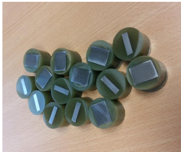
Fig. 2.13. Work pieces after surface polishing
