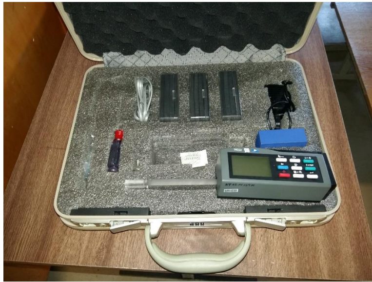
Fig. 2.21. Surface roughness tester TR220
