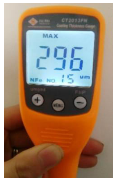
Fig.7.3 Digital paint thickness gauges meter
