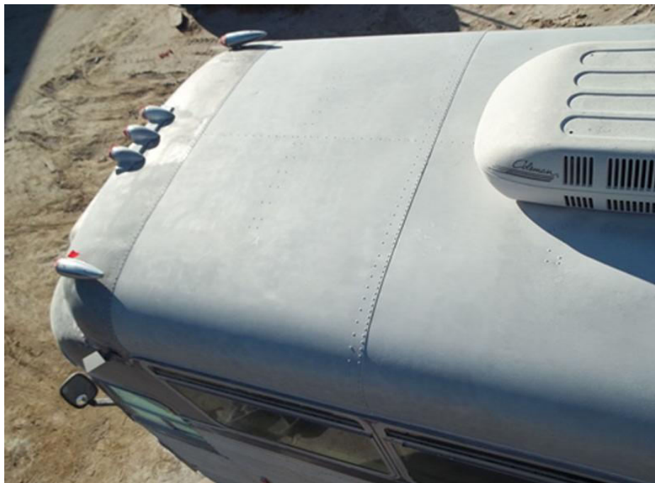
Fig.3.2 Surface after blasting
