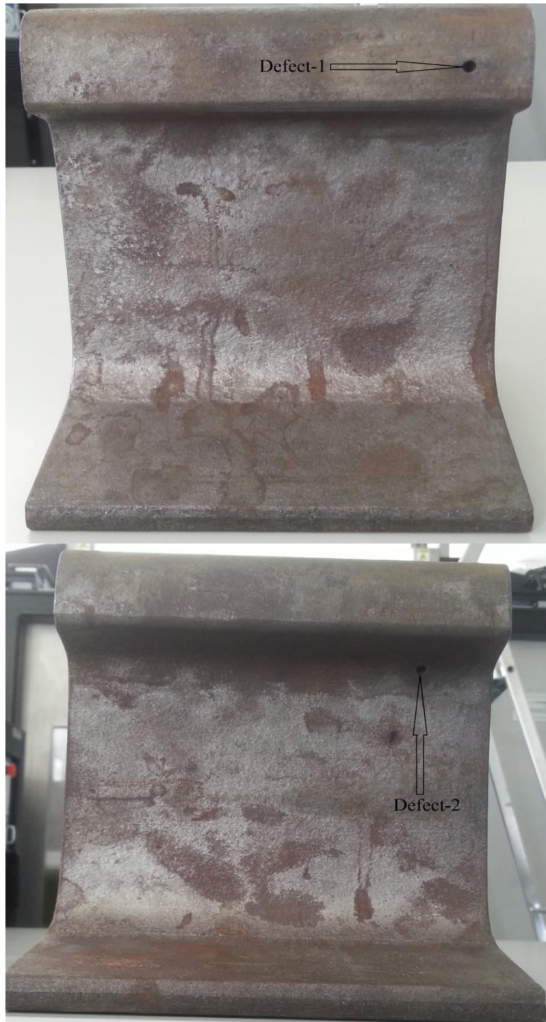
Fig.2.2. Location of defects in the test sample
