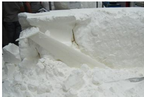
Fig. 3.2 Example of powder accumulations [28]
