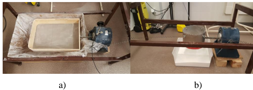
Fig. 4.8 Sieving prototypes: a) early sieving assembly, b) later sieving assembly
