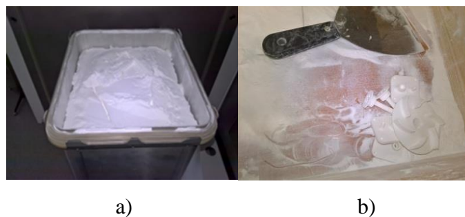
Fig. 4.9 Post-processing; a) container after printing, b) powder removing from parts
