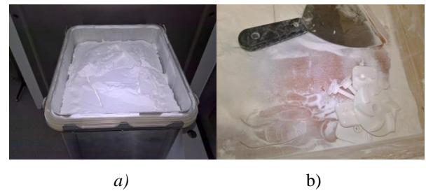
Fig. 1 Post-processing; a) container after printing, b) powder removing from part
