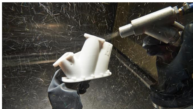
Fig. 1.10 SLS printed part cleaning using bead blasting station [24]
