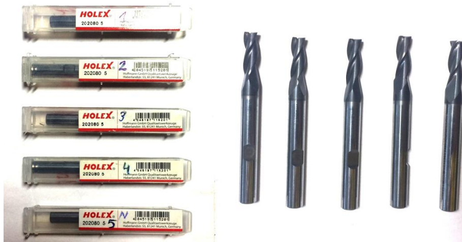
Fig. 2.3. \varnothing 5 diameter cutters examples
