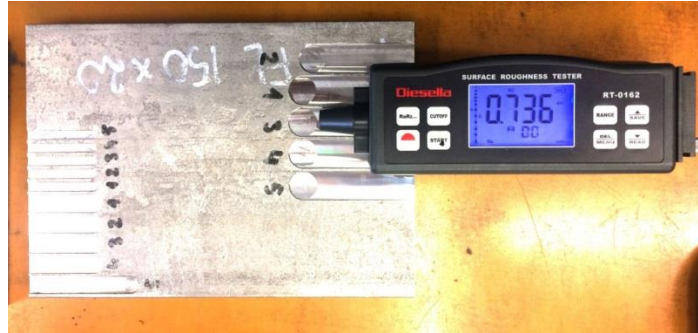
Fig. 2.10. Milled surface roughness measurements procedure
