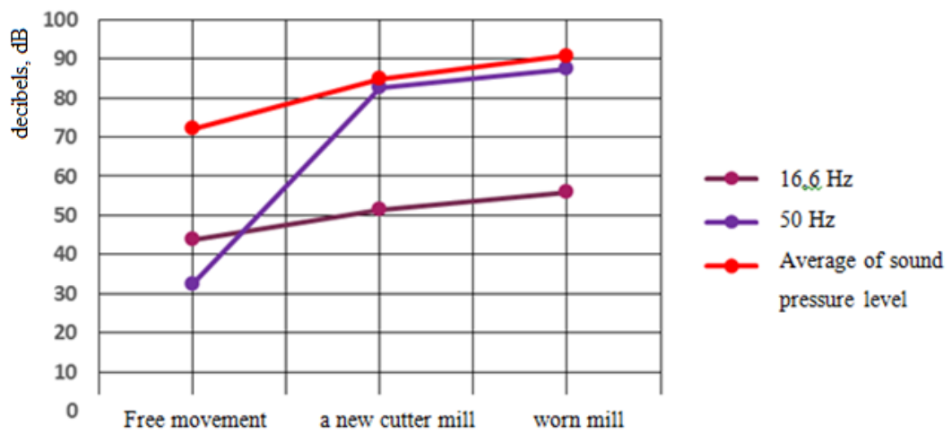
Fig. 3.19. CNC machine sound level dependence from milling cutters quality
