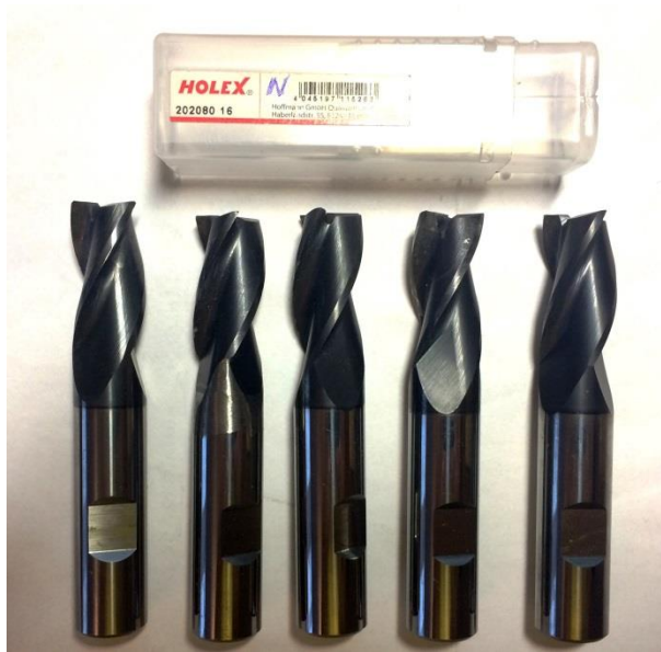
Fig. 2.4. Ø16 diameter cutters examples
