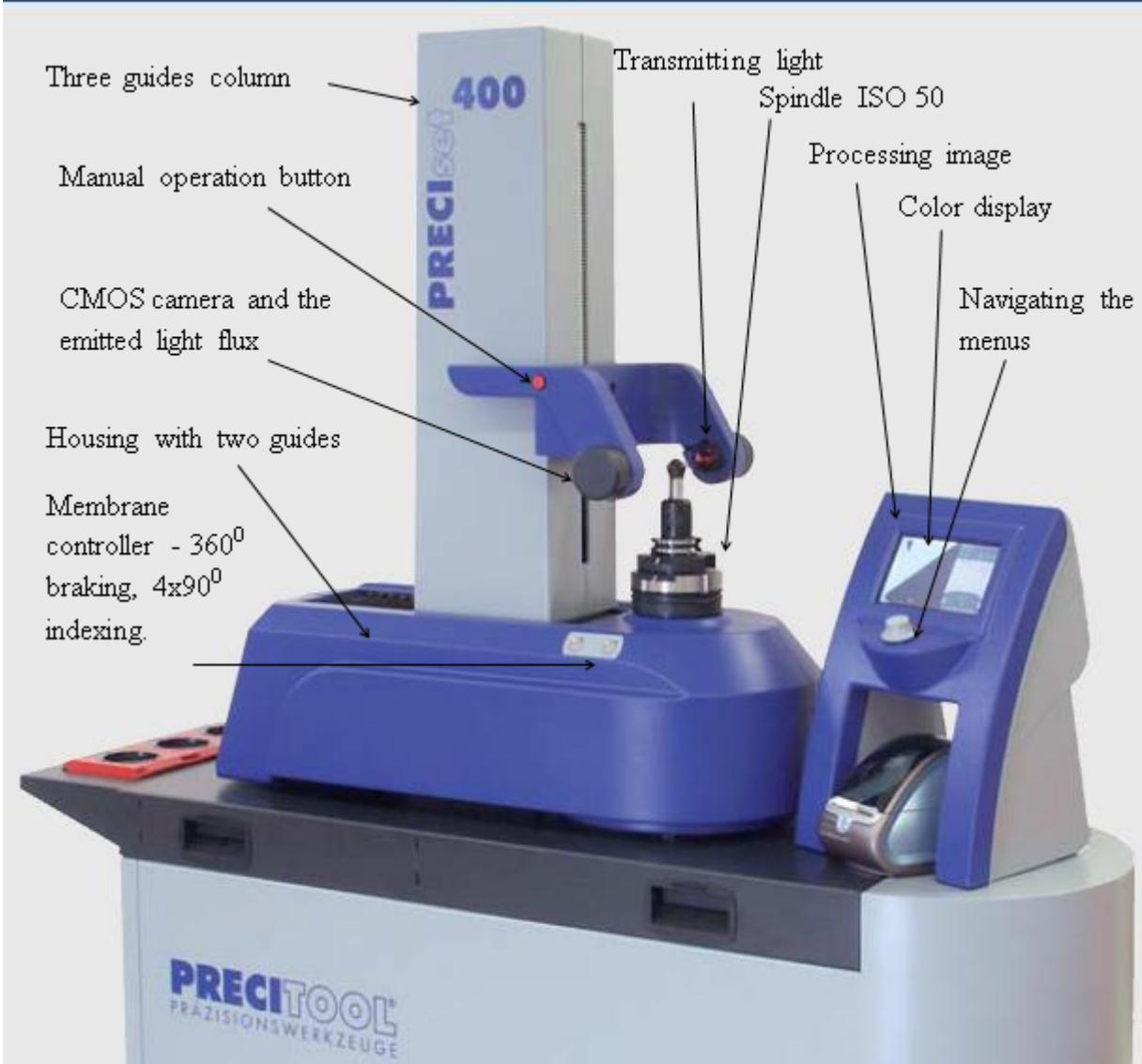
Fig. 2.5. Measuring machine Precitool set basic 400 [21].
