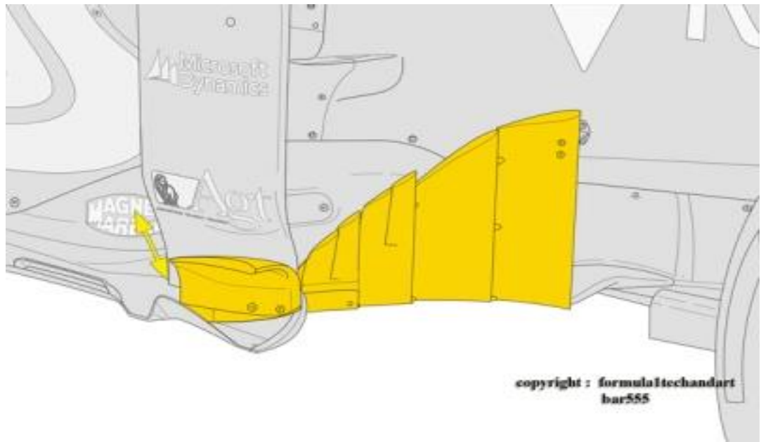
Fig-9 Barge board [17]
