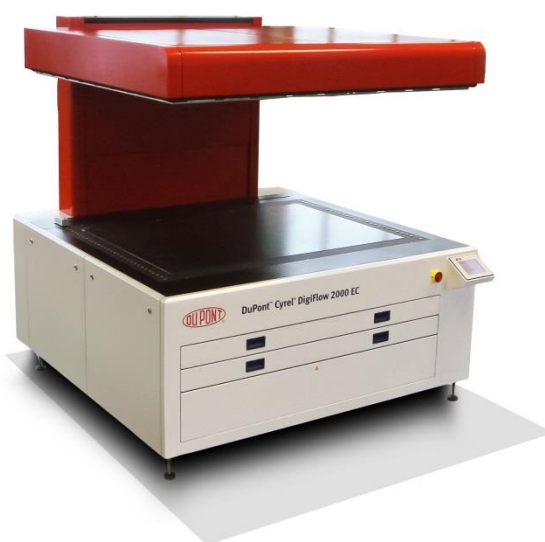
Fig 13.3 Exposure equipment- Dupont Cyrel DigiFlow 2000 EC and technical characteristics
