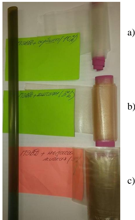
Fig. 5.2. The outer view of biodegradable materials: a) LDPE+ sorbitol 10 % ,b)LDPE+ Chitosan 3 %,c) LDPE+ Molasses liquid 3 %
