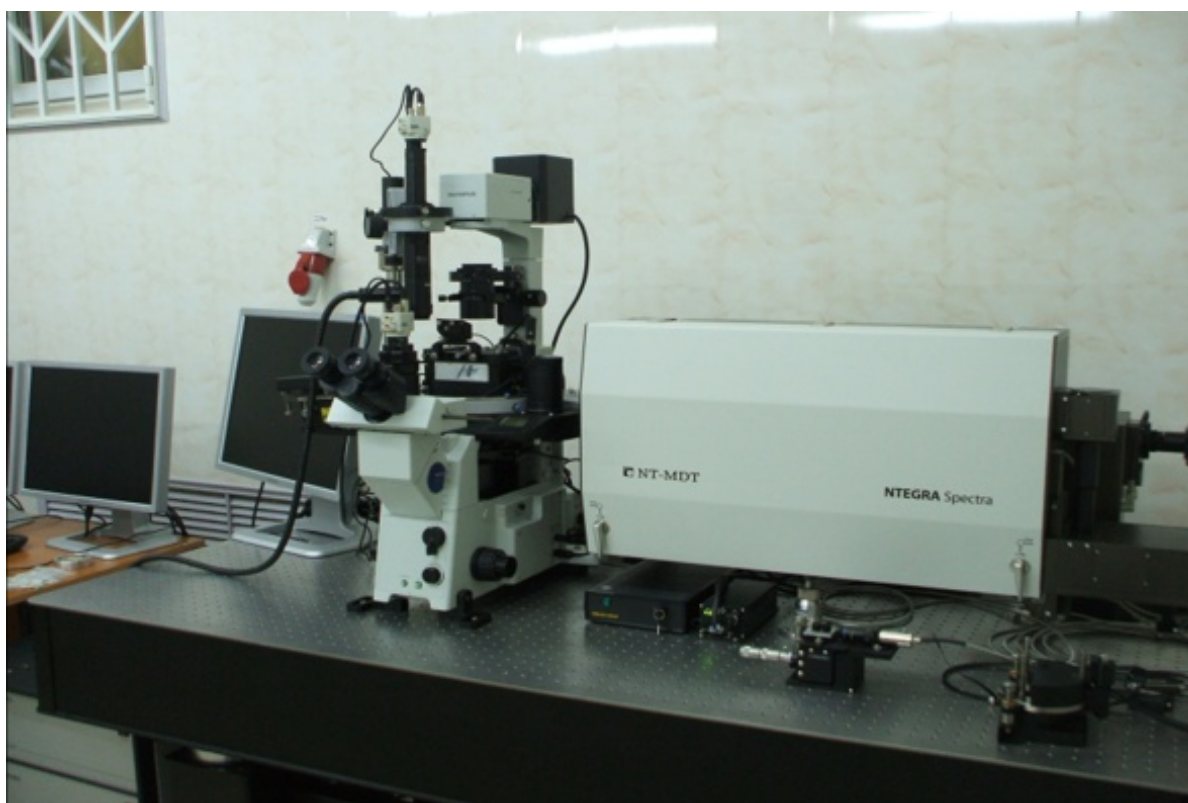
Fig. 2.4.1. General view of Confocal Raman spectrometer Solver Spectrum (NT-MDT, Russia)
