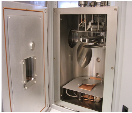
Fig. 2.2.5. The working chamber of the E-Beam Evaporator (PVD 75)
