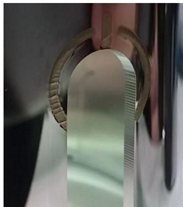
Figure 2.5 Laser engraving crack scrap on FOT-C
