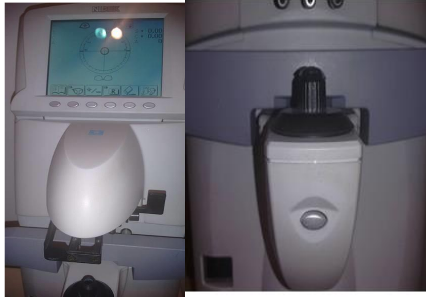
Fig.24. Lensmeter display data when examined contact lens.
