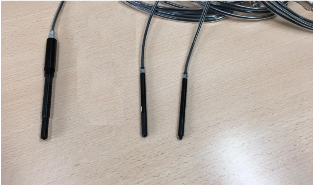
Figure 21. The ion chambers used for this project. Left to right: A19MR ion chamber, A1SLMR ion chamber and A26MR ion chamber.
