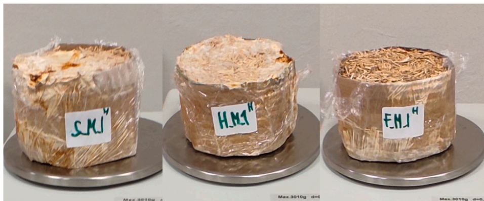
Fig. 2. Flax (F.M.1),-hemp (H.M.1) and wheat (S.M.1) composite samples with fungal mycelium as a binder.
