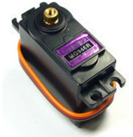
3.15 pav. Servo pavara TowerPro MG945R [15]
