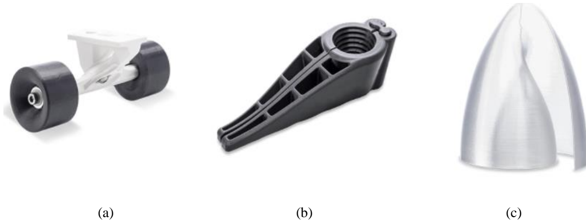
Figure 22 PC printed examples, (a)Stable dimension, (b)Tough and strong, (c)Optically translucency [25].
