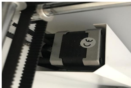
Fig5: Stepper motor in Ultimaker 2+
