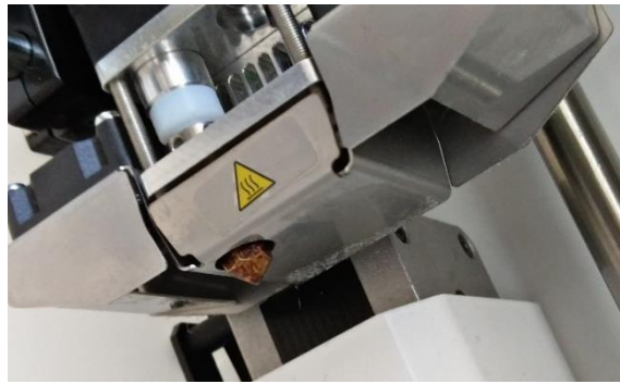
Figure 12 Ultimaker 2+ head nozzle located region
