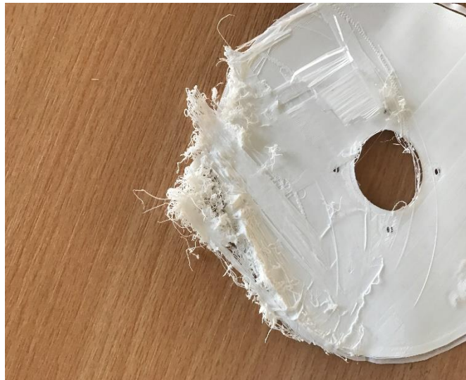
Figure 9 Printed parts in where we can see bad prints and under construction problems
