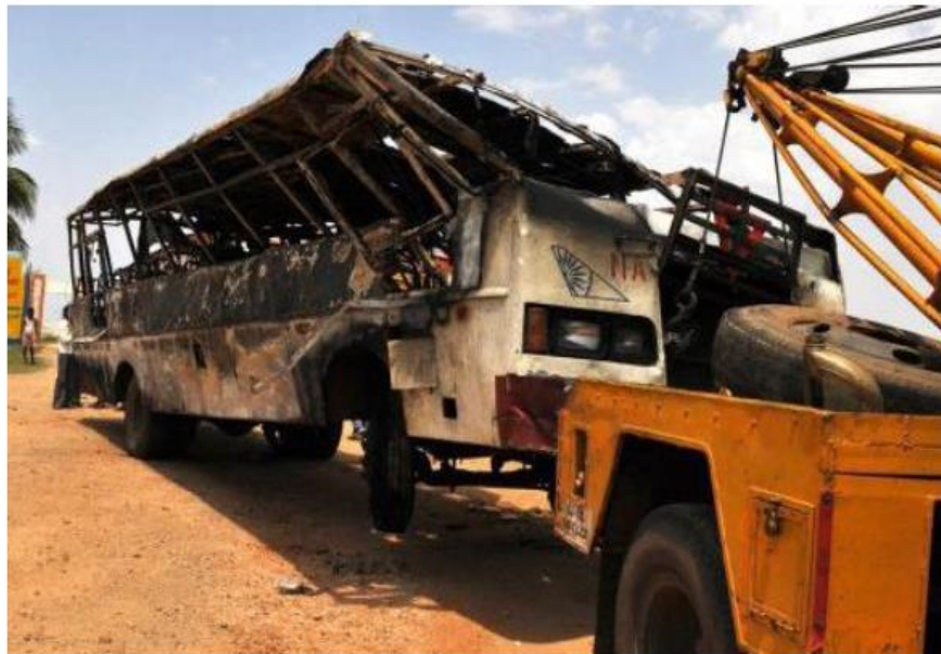
Figure 1. 1 Damaged Bus Structure due to Rollover and Fire [2]
