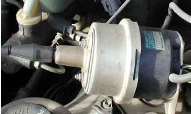
Figure 3. 3 the electronically-controlled vacuum actuator that controls the throttle
