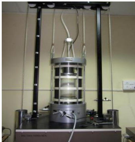
Figure 25 An image of HCT apparatus with specimen inside HCT cell (Singh, Kandasami and Murthy 2017)
