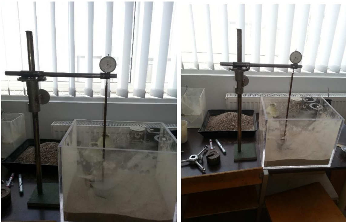
Figure 51 actual model footing type 1 and 2
