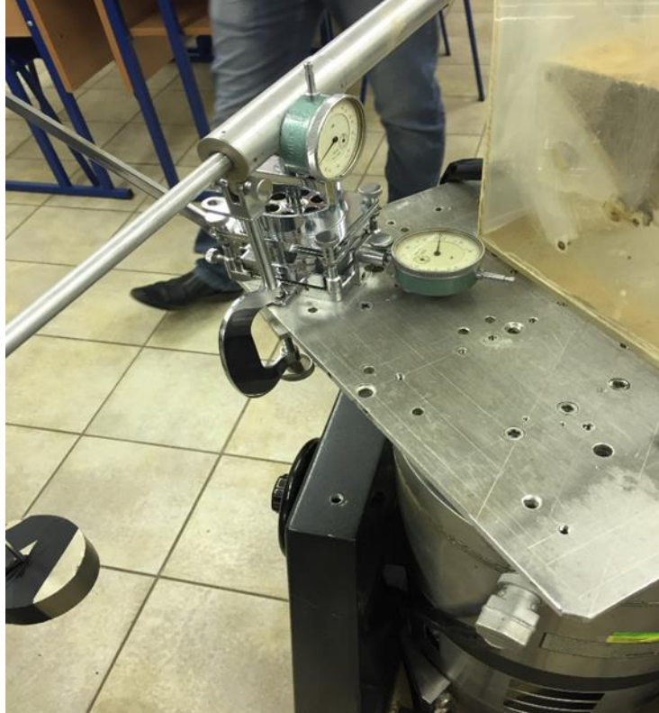
Figure 42 vibration table with varying cyclic loading
