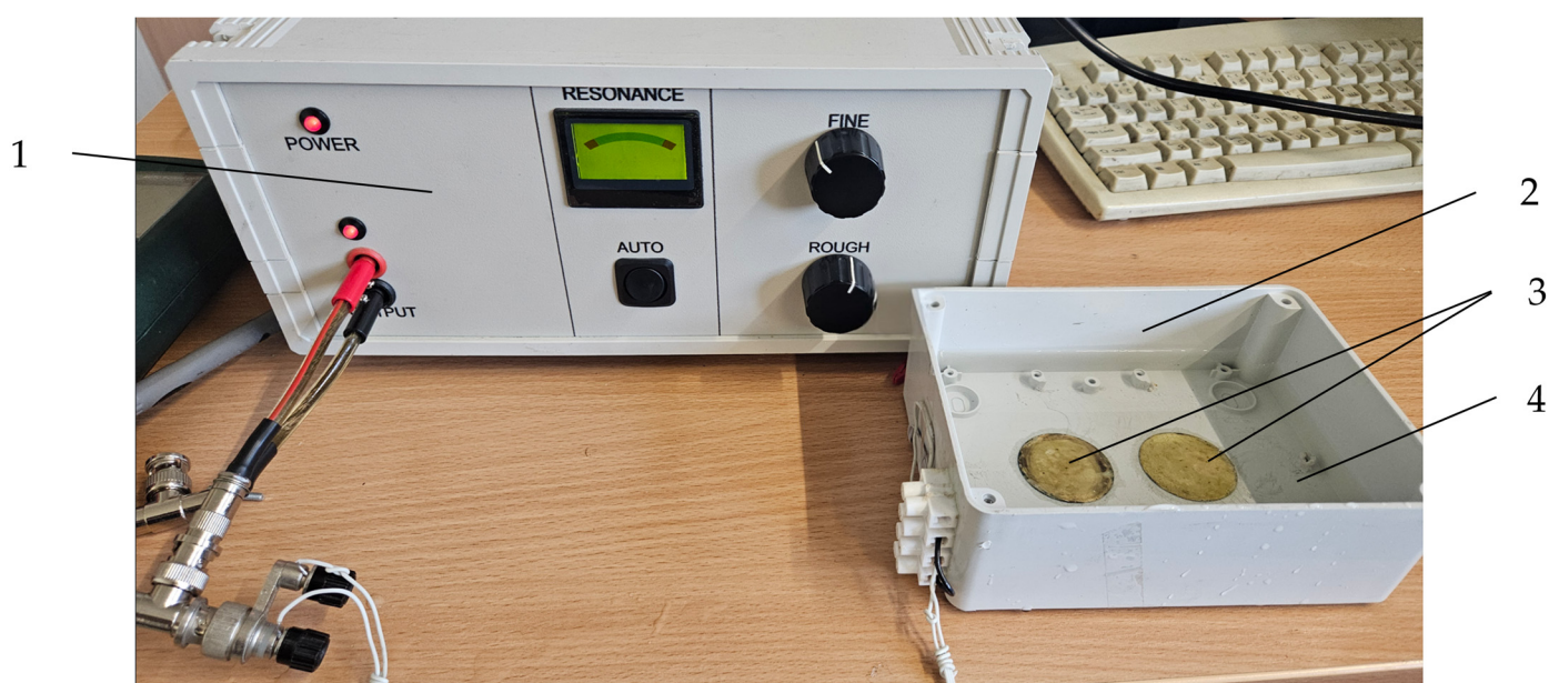
Figure 8. Ultrasonic bath with signal controller: 1—signal controller; 2—ultrasonic bath; 3—piezo elements; 4—distilled water.
