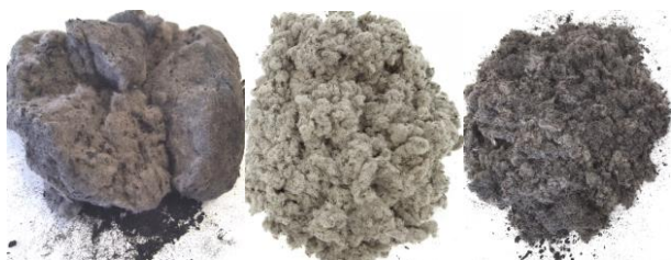
Figure 1: Investigated textile waste: a – raw textile waste from recycled tires, b – marginally polluted, c – highly polluted
