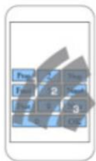
Figure 15: Areas reachable by the thumb with little help from supporting fingers.
